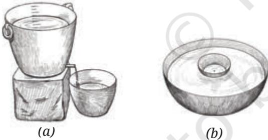
Fig. 8.2 A water clock (a) Water flowing out-type
